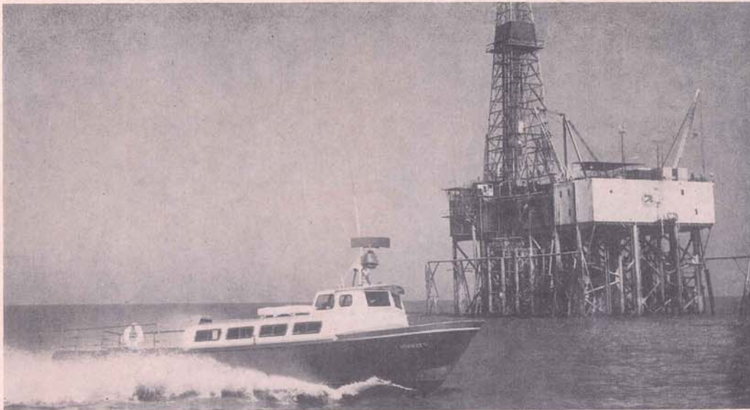
An all aluminum 50 foot crewboat operating in the Gulf of Mexico off the Louisiana Coast, built to the order of the George Engine Company in a Louisiana shipyard, and powered by a pair of General Motors Series 71 V-8 engines which give it a speed in excess of 30 miles per hour. The George Engine Company on the Harvey Canal is the world's largest distributor of General Motors marine diesel engines.
