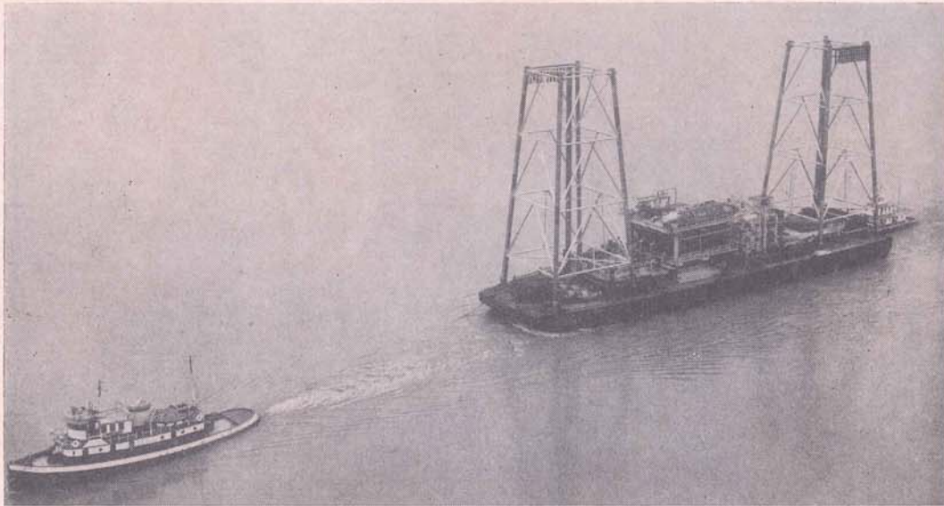
Harvey based J. Ray McDermott tug "Rosalie E" and barge "Ven Mac #2" shown departing from McDermott Fabricators yard at Bayou Boeuf for direct tow to Lake Maracaibo, Venezuela. Loaded on the barge are two aluminum drilling platforms and a 100,000 barrel per day production flow station built by McDermott for the Venezuelan Sun Oil Company.
