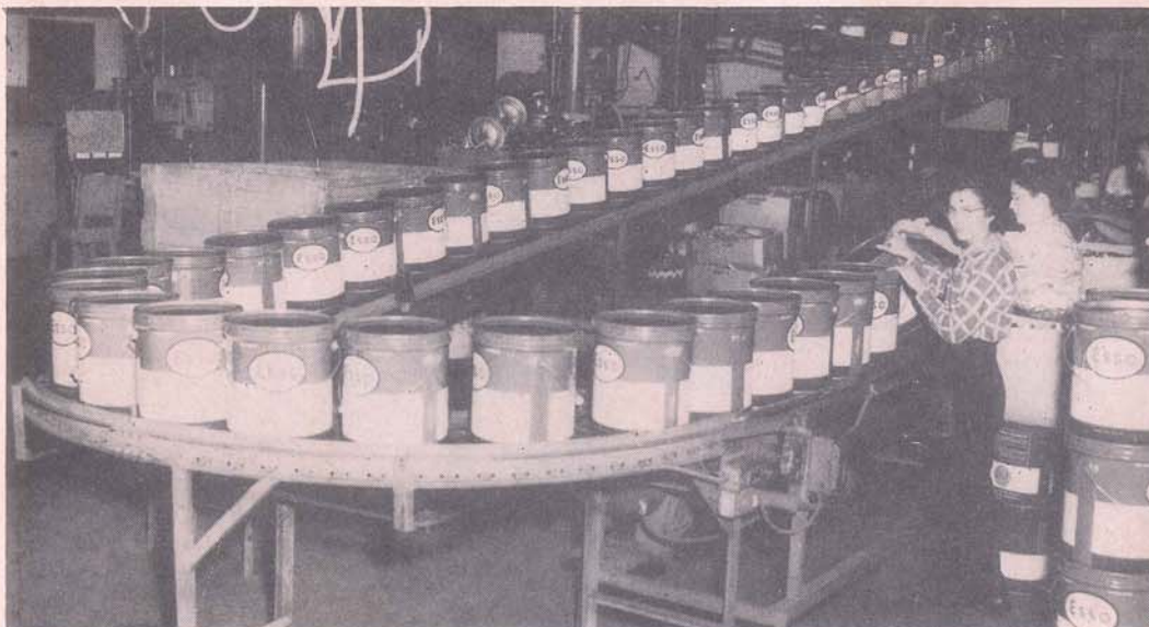
At the Jefferson Parish plant of the Rheem Manufacturing Company, the world's largest producer of steel containers, already lithographed 5-gallon pails for Esso, are shown coming off the production line to where handles are hooked on and pails ascend power conveyor to box car for shipping.
