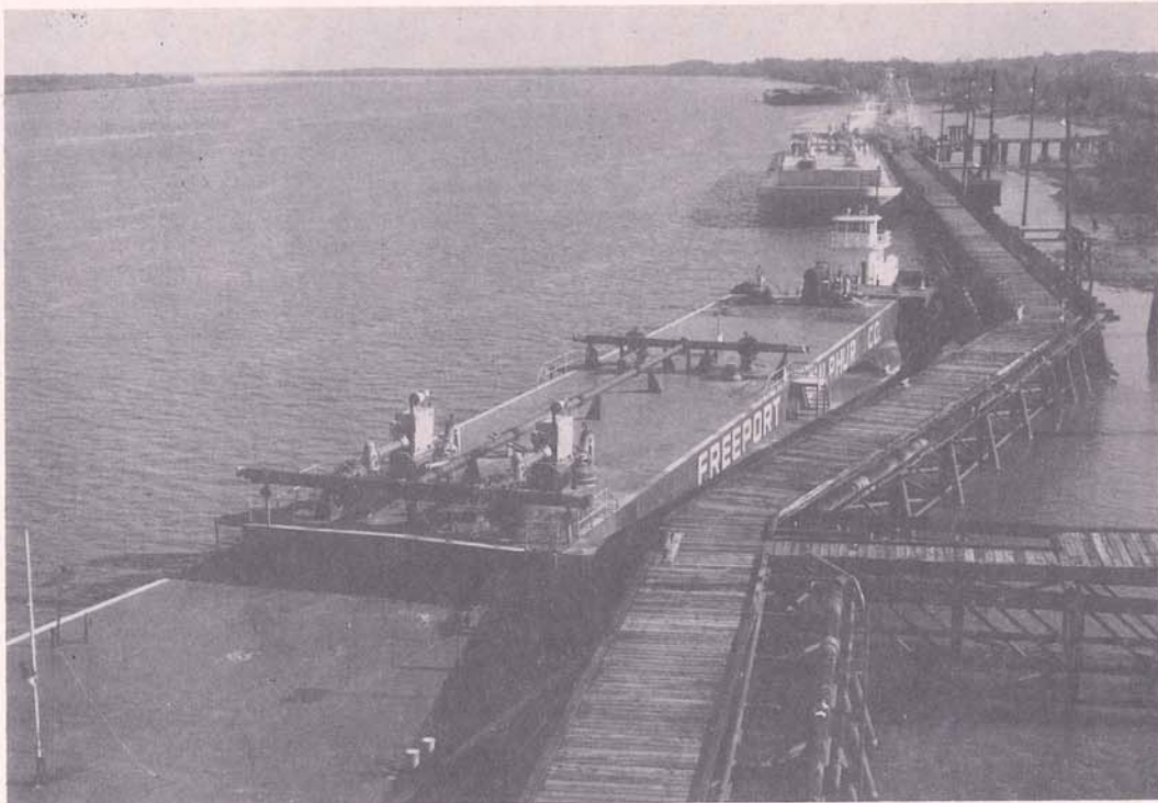
A huge liquid sulphur barge (background) takes on a load of hot molten sulphur at Freeport Sulphur Company's facilities at Port Sulphur while a sister barge stands by in the foreground. These barges ply the Mississippi, Illinois and Ohio Rivers to serve liquid sulphur storage terminals as far as 1,900 miles from Port Sulphur. The liquid sulphur stored in the barge's two heavily insulated tanks is kept at 275 degrees Fahrenheit by hot oil circulating through coils.
