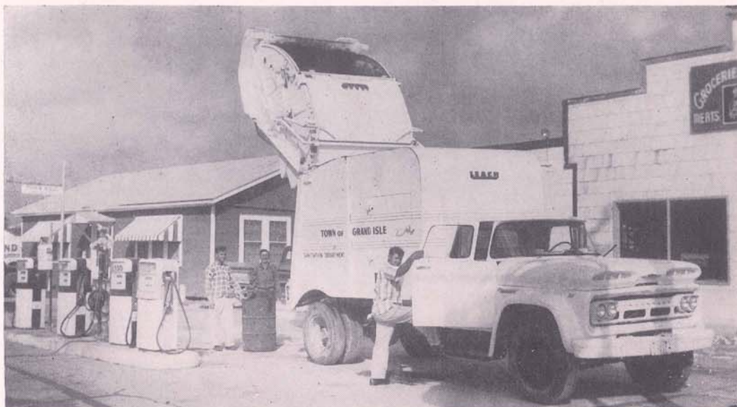
Grand Isle's new 16 cubic yard, Packmaster type Garbage Truck operated by, left to right, Lamsey M. Chermie, Hilton P. Besson and Hirvin M. Barthelemy.
