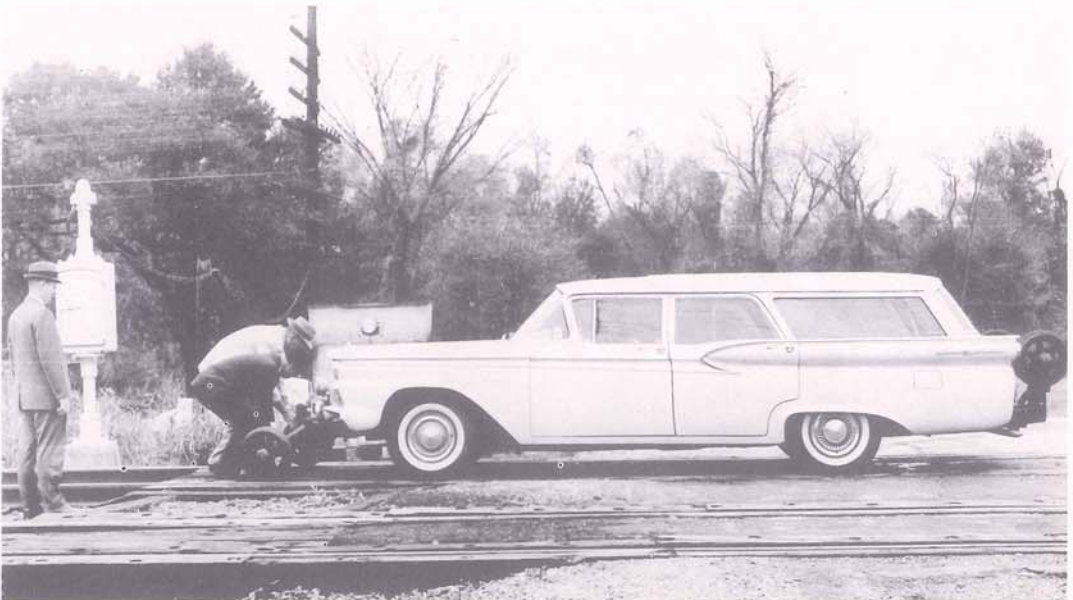
Engineering and traffic officers of the Illinois Central Railroad prepare to drop the guide wheels of the "hi-railer" in preparation for making an inspection tour of the Harahan Industrial District.
