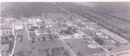
The Jefferson Parish plant of the $100 million American Cyanamid operation near Waggaman on the Mississippi River, the sixth largest chemical company in the world. Here natural gas is converted into acetylene and then into acrylonitrile which is in turn converted later and at another plant, into Creslan, a new and important synthetic fiber.
