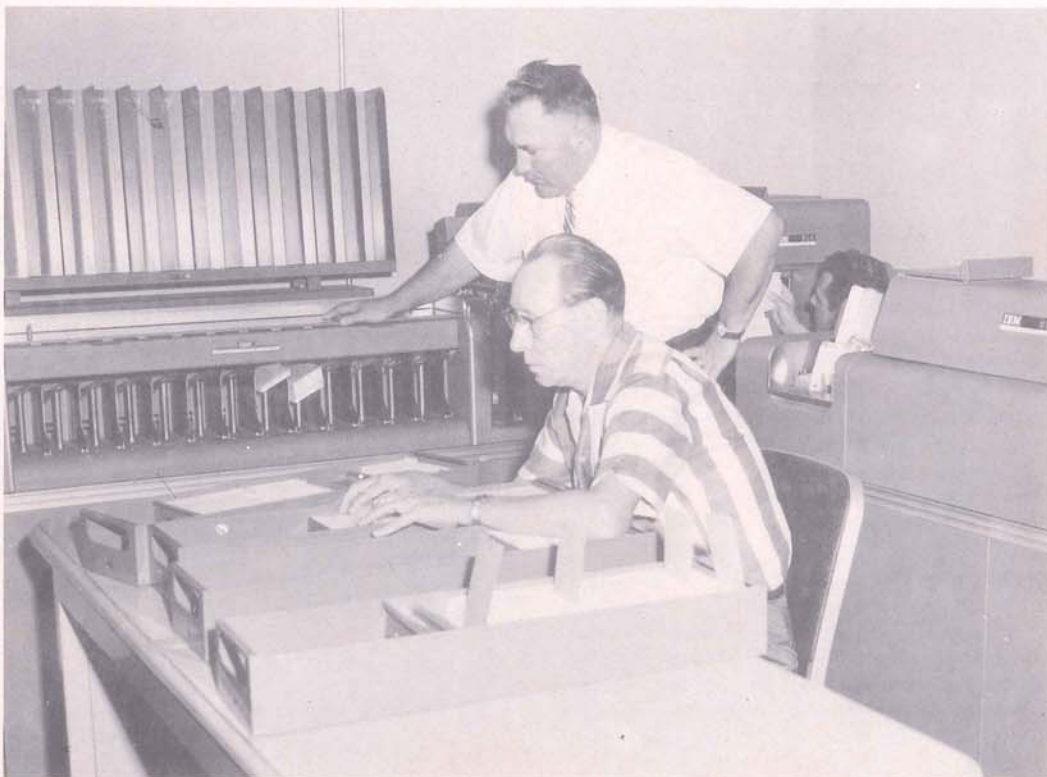
In this modern world of computers and electronic accounting systems are shown three Deputy Assessors of Jefferson Parish. One is working the IBM Card Sorting Machine, one is consulting file drawers and in the background a third deputy is operating the 407 Accounting Machine.
