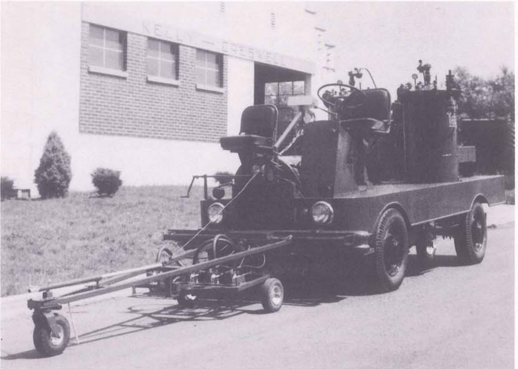
The new Kelly-Creswell Model WV-4 Striper of the Traffic Division of the Jefferson Parish Safety Department, capable of striping ten miles of four inch line per hour.
