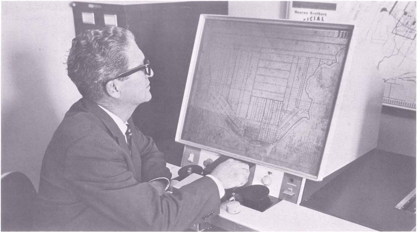
Arthur Acosta operates printer-reader machine which can reproduce subdivision maps up to 18 by 24 inch size from microfilm masters. Mortgage cancellations are processed on third floor.
