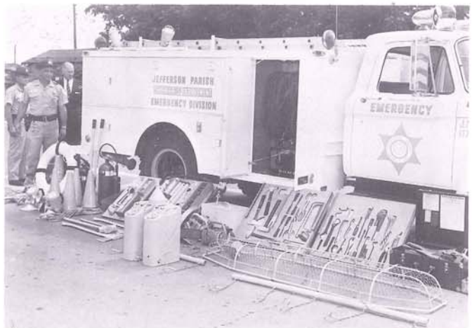
New emergency rescue truck responds to all emergencies. It contains portable power tools, emergency lighting equipment, complete first aid and life saving gear and portable generators.
